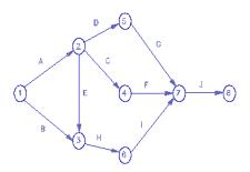
Fig.1: CPM Network Diagram
